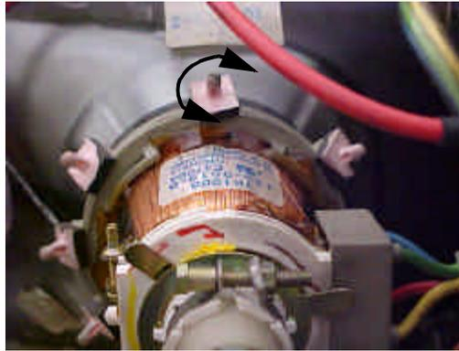
Geometric distortion so large that it can't be corrected with rotating these magnets is indicative of a serious problem, generally with the yoke or flyback.
